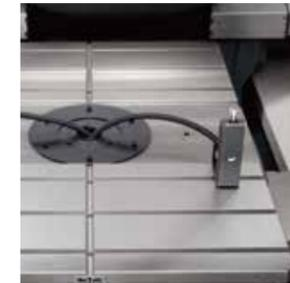
**Tool breakage detector, touch type**
