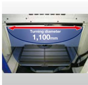
**Turning diameter enlargement (R450Xd1: ø1,100, R650Xd1: ø1,300)**
