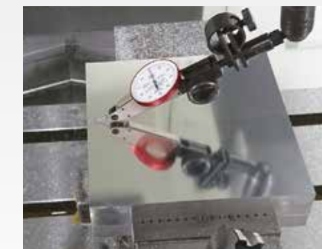
DYPEC ® mirror milling with ball end mill
